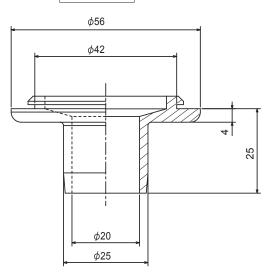
The outdoor unit is provided with several holes for drainage at the bottom to ma easier. The drain socket is used to close the unnecessary holes and centralize
