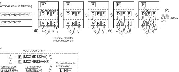
Be sure to attach each screw to its correspondent terminal when securing the cord and/or the wire to the terminal block. Make earth wire a little longer than others. (More than 35 mm)
