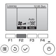
Press the F2 button to go through the fan speeds in the following order.
