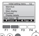
Move the cursor to the "Contrast" with the F1 or F2 button, and press the SELECT button.
