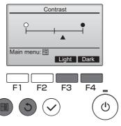
Adjust the contrast with the F3 or F4 button, and press the MENU or RETURN button.
