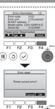
Press the F4 button or the ON/OFF button to reset the error that is occurring.
