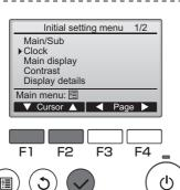
Move the cursor to the "Clock" with the F1 or F2 button, and press the SELECT button.
