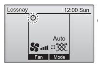
(1) will appear on the Main display when the On/Off timer is enabled.
