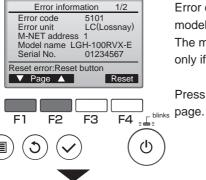
Error code, error unit, M-NET address, unit model name, and serial number will appear. The model name and serial number will appear only if the information have been registered.
