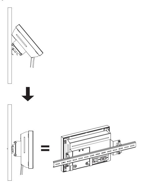
Removing the AE-200/AE-50 from the DIN rail
